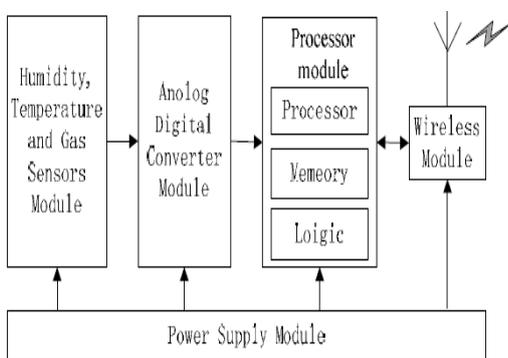
Fig. 2 The block chart of sensor node
