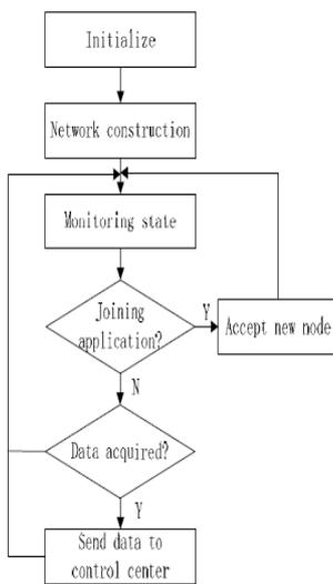
Fig. 3 The software flowchart of sensor node
