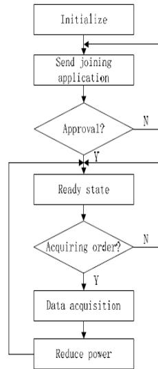
Fig. 4 The software flowchart of sink node
