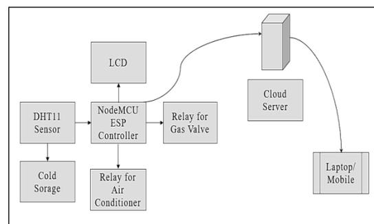
Fig 1. Block diagram for proposed idea
