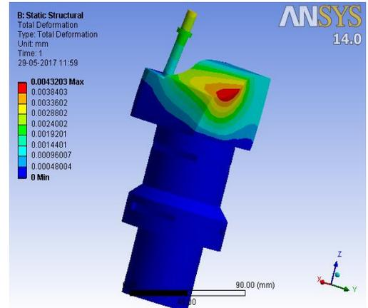
Fig 5 Total Deformation
