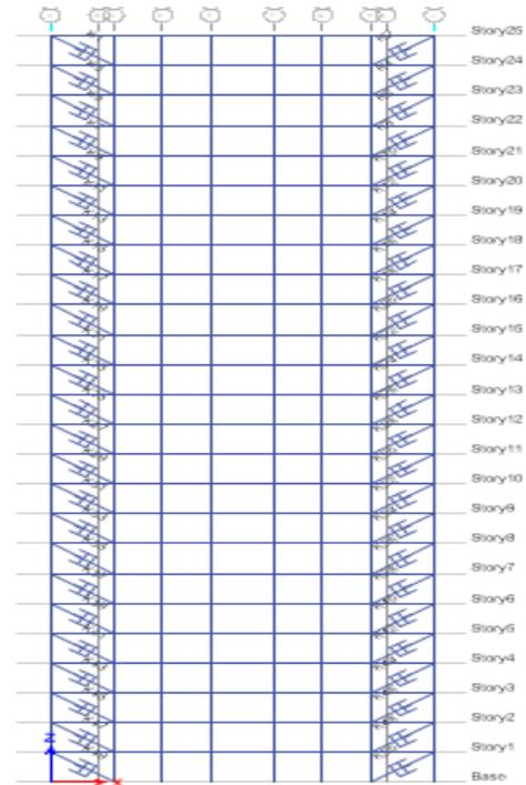
Fig.3- FVD at exterior corner Elevation in YZ plane
