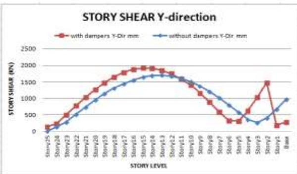
Graph 10: Storey shear in Y direction for Static method
