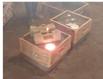
Fig 4: Molten Cast Iron poured and holes made for internal chilling at Deepshikha Castings Pvt. Ltd. Nagpur, India
