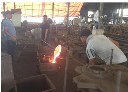
Fig 1: Pouring the molten Cast iron into the mould at Deepshikha Castings Pvt. Ltd., Nagpur, India
