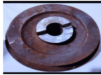
Fig 2: Cast iron Machine Pulley Specimen By Normal Process At Deepshikha Castings Pvt. Ltd., Nagpur, India
