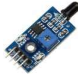
Fig No.07 Fire sensor
