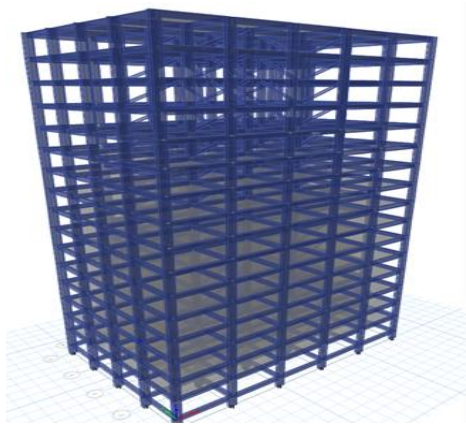
Fig.6- 3D view of G+15 RC frame building with inner diagonal steel bracing
