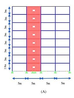
Figure 3: Steel Structures with Coupled Shear Wall with Opening Dimensions Changes for Nonlinear Analysis in ETABS Program with Grid Line D a) Opening Dimensions 1x0.9 b) Opening Dimensions 1x0.6 c) Opening Dimensions 2x0.9 d) Opening Dimensions
