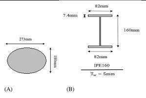
Figure 1: Sections of Steel Structures with Coupled Shear Wall with Opening Dimensions Changes in ETABS Software A) 3IPE18 B) IPE160
