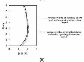
Figure 8: Comparison of maximum measure of displacement between frame with coupled shear wall with opening dimensions of 1x0.6 and 2x 0.9 a) In far-fault records b) In near-fault records
