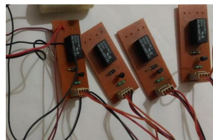
Fig 3- 3D View of Relay section
