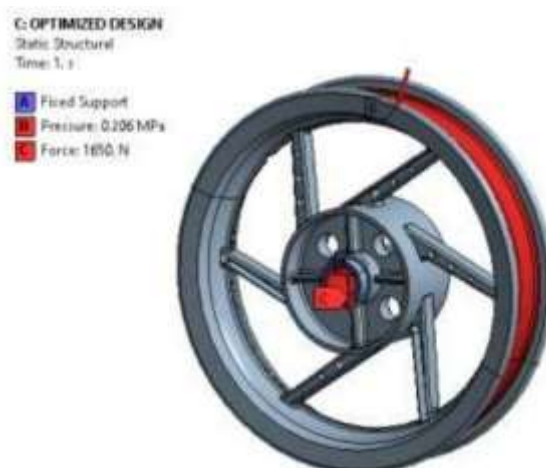
Fig 11- Bouandary condition on optimized design
