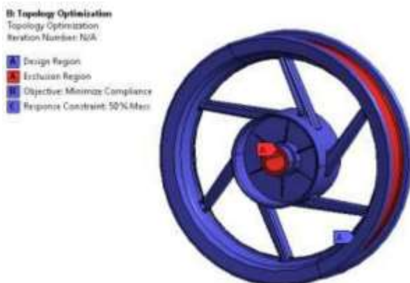
Fig7-Boundary condition of topology optimization
