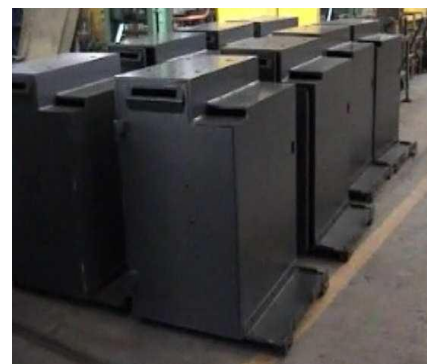
Fig-3 ATM Bodies after Welding
