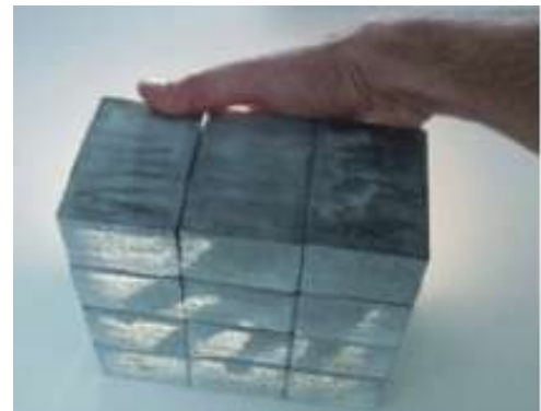
Fig 1: Picture of LiTraCon light transmitting concrete
