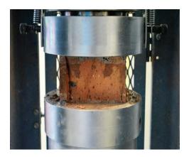
The UTM was using the tests. The compressive strength of bricks. After the curing period gets over bricks are kept for testing. To test the specimens, the bricks are placed in the calibrated compression testing machine of capacity 3000 KN (Kilo Newton) and applied a load uniform at the rate of 2.9 kN/min. By obtaining the maximum load shall be taken as failure of load with specimen fails to produce
