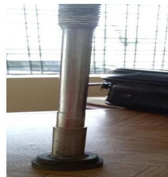
Fig(E)-ROD USED FOR INNER DIAMETER OF BUSHES
