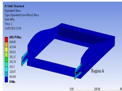
**2) Maximum Bending Stress for ECE R-17 Backrest Moment Test on Contact between the Vertical Member and Connector of Seat Back Frame**
