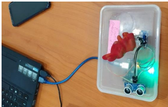
Fig 7-Implementation of Ultrasonic Radar System
