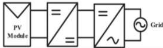
(b) Two stage inverter
