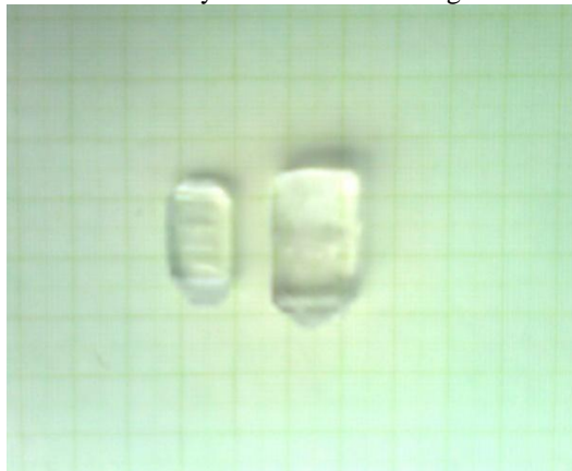
Fig.1. Grown crystals of BGSN mixed ADP
