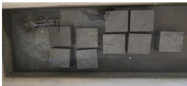
Fig 4.2: Cubes for curing
