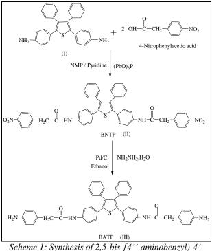
*Scheme 1: Synthesis of 2,3-Dis-[4 -aminobenzyl)-4 benzamide]-3,4-diphenyl thiophene (BATP)*
