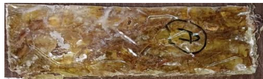
Fig.1 Sample1 (80 PLA -20 coconut shell powder- 0 Ammonium polyphosphate)
