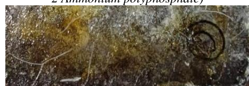
Fig.4 Sample (77 PLA - 20 coconut shell powder - 3 Ammonium polyphosphate)
