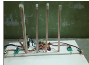
Fig 3.4.5- And Step by step Next Street Lamp start Glow Brighter as per calculated Speed of the vehicle/object that is detected by the Microcontroller, using IR sensor. And Street Light again goes into a DIM condition.
