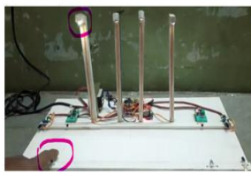
Figure 3.4.3- 1 st IR Sensor sense Vehicle and Microcontroller start Calculating Speed of the Vehicle Figure 3.4.4- As soon As 2 nd IR Sensors Sense the Light glow brighter, before object is reach. As per speed of the vehicle.
