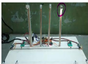
Fig 3.4.5- And Step by step Next Street Lamp start Glow Brighter as per calculated Speed of the vehicle/object that is detected by the Microcontroller, using IR sensor. And Street Light again goes into a DIM condition.
