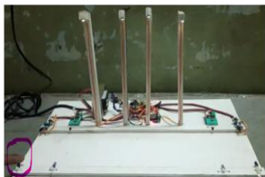
Figure 3.4.3- 1 st IR Sensor sense Vehicle and Microcontroller start Calculating Speed of the Vehicle Figure 3.4.4- As soon As 2 nd IR Sensors Sense the Light glow brighter, before object is reach. As per speed of the vehicle.
