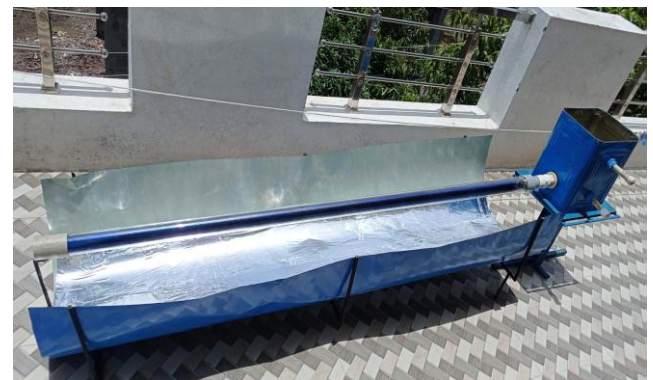
Fig. 1- Parabolic Solar Water Heater System
