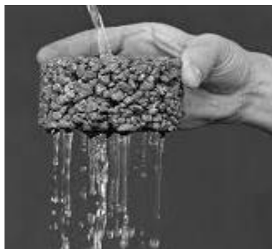
Figure 1: Pervious concrete sample in the passage of water.
