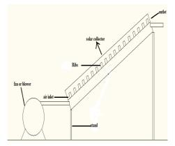
This is the purpose setup of solar air heater having the flat plate collector installed and the ribs with the absorber plate for forced convection the fan is provided at the inlet of the test section of the solar air heater .This is used to test the heat transfer effect during the forced convection as the fan is used at the inlet of the test section.
