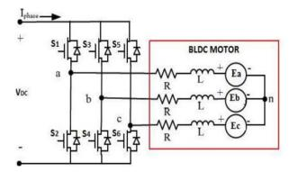
Fig.1 Equivalent circuit of a BLDC motor connected to an inverter [3]
