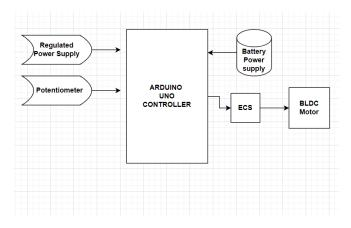
Fig.4 Proposed Schematic Diagram of Hardware Development [4]
