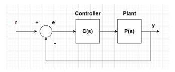
Fig. 7 Feedback control system [4]
