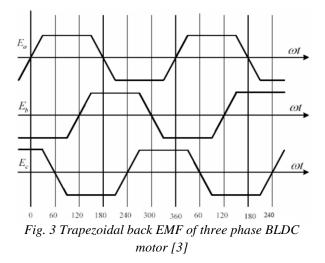
In this study, they assume that hall sensors are being used to gather the rotor data. The real rotor position is sensed by the 120-degree-apart Hall position sensors [3].
