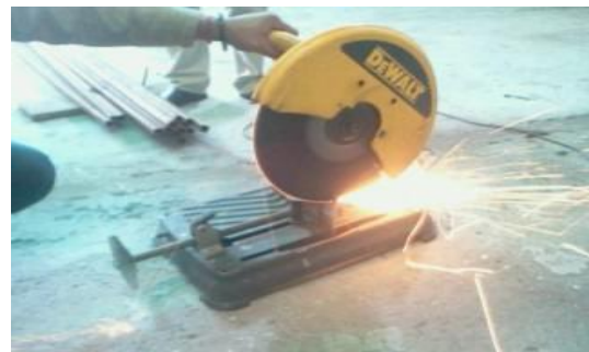
Fig 3: MS Plate cutting setup.
