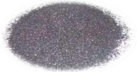
Fig 3.1 Image of copper slag used in the concrete
