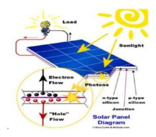
Fig. 2 - Solar Panel Diagram
