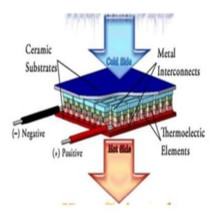
Fig.3 - Operating principle of thermo-electric module
