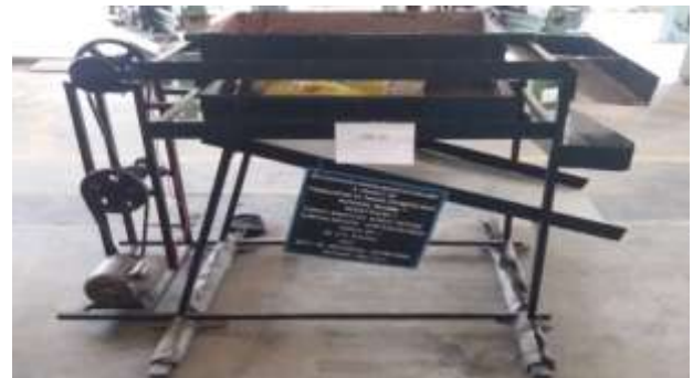
Fig.1: Fabricated Photo of sand filter
