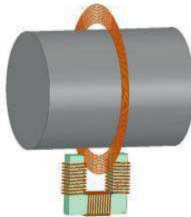
Figure 1: Schematic diagram of U-type coupling structure WPT system.
