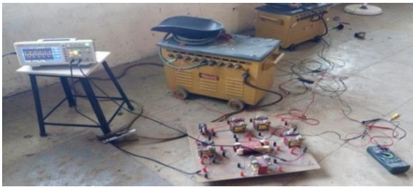
Fig 1:- System Set Up with Transformers PT's
