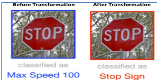
Fig.3- A stop sign that underwent modification so that the ML model could identify it as a speed limit sign.
