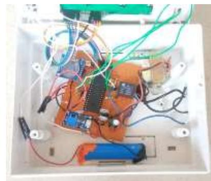
Figure 6: Automatic security light control system setup
