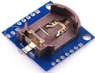
Figure 4: RTC module
