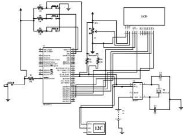
Fig. 5- Schematic Circuit of the Security Light Control System
