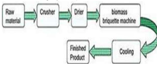
Fig. No. 1.1 Preparation Method of Composite Briquettes From Agriculture Waste.
