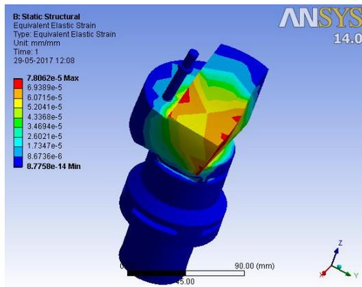
Figure 7: Strain distribution in fixture.
