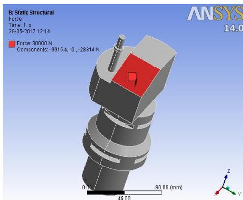
Fig 4 force on fixture
