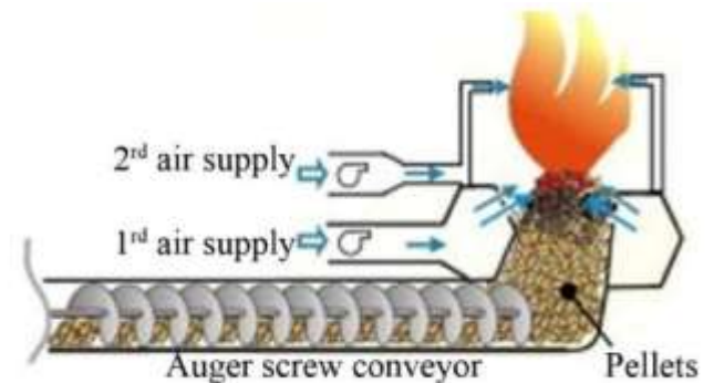
Fig.2. The Rectangular Shaped Pellet Burner [7]
