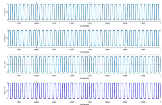
*Fig.4-Phase shift pulse of Dual active full-bridge DC-DC converter*
