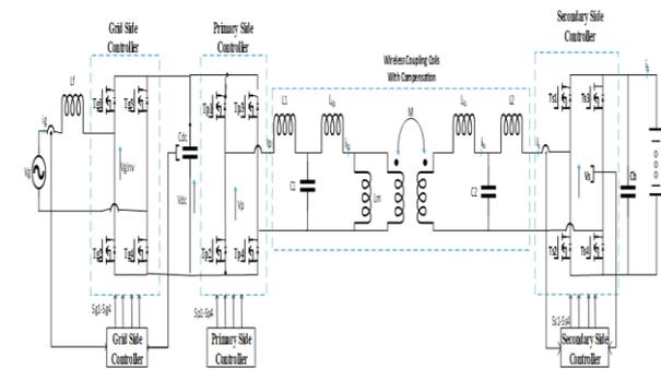
*Fig 1: Grid Connected BD-WPT System*
