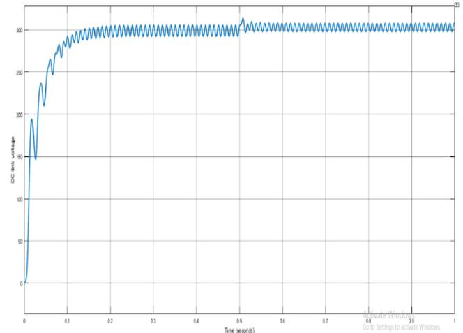
*Fig 7: DC link voltage after controlled rectifier using a PI controller*
