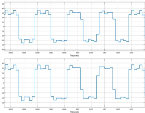
*Fig 5: Primary and Secondary voltages of high frequency transformer*
