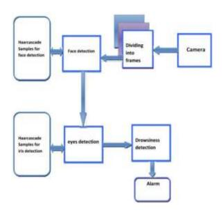
Figure 3.1 System Architecture
