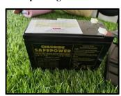
At the time of power shortage, the battery storage bank is used to store the power as a backup supply in case of emergency. In this paper, lead—acid battery is used to store the power. The battery specifications are 12 v, 7 Ah used in the project.
