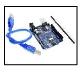
This is an electronic controlled board which is used to communicate between Human and Machines by using Coding. In the paper Arduino Uno R3 is used to give directions to the RFID Module i.e. This will scan card by RFID and if card is valid then it will start charging the vehicles otherwise this will ring an indicating buzzer. Therefore, Arduino is used to defined the identity of the electric vehicles.
