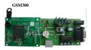
SIM300 is a Tri-band GSM/GPRS engine that works on frequencies EGSM 900 MHz, DCS 1800 MHz and
