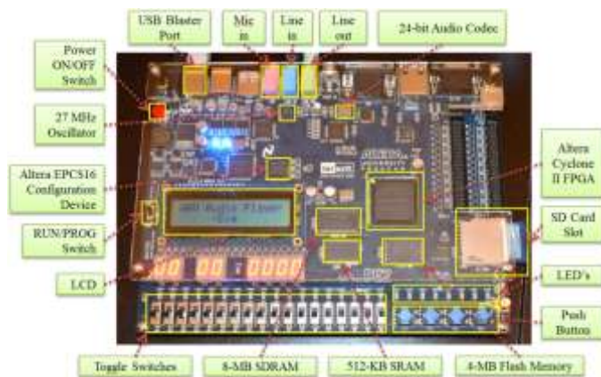
Figure 6 . Altera DE2 Board Components and Interfaces
