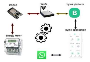
Fig: 1 Architecture of Smart Energy Meter System
