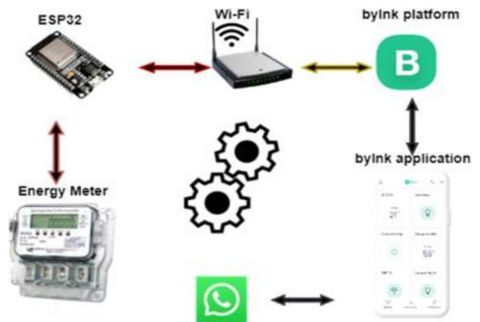
Fig: 1 Architecture of Smart Energy Meter System
