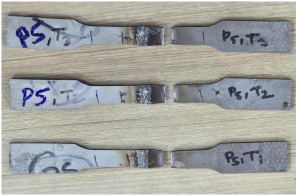
Fig 4: Fractured tensile sample
