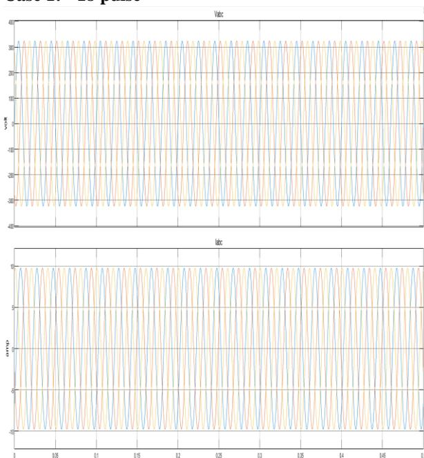
Figure 7:-Grid voltage and current waveform at LG fault condition with STATCOM
