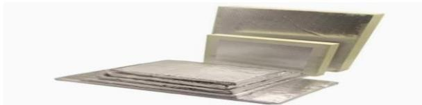
**Figure 5- Vacuum Insulated panel [37]**
