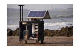
Fig. 6 Solar-Powered Seawater Desalination System with RO and UV Purification
