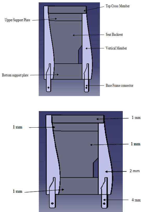
Fig.1 Nomenclature of Seat Backrest Frame Fig.2 Shell Thickness of Seat Backrest Frame
