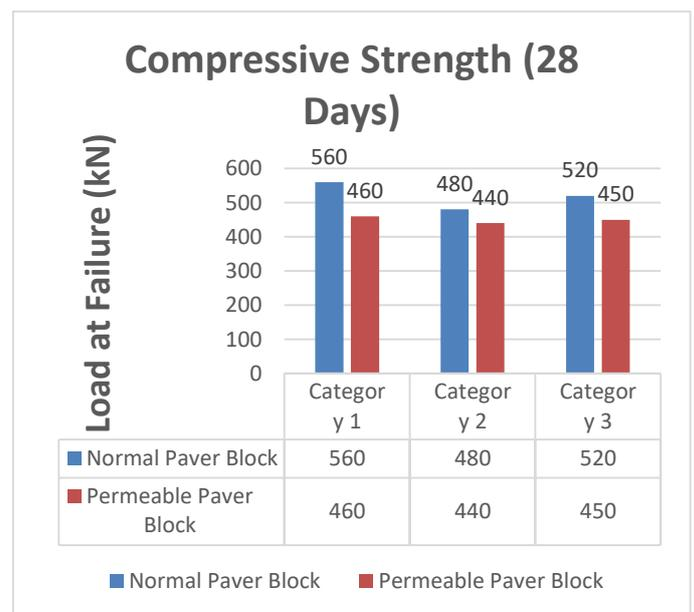
Fig.1.3-Compressive Strength (28 Days)
