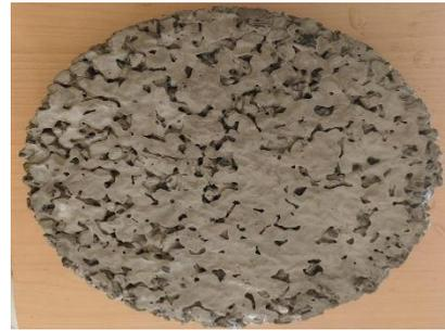
Fig. 1.1- Permeable Concrete Block (Circular)
