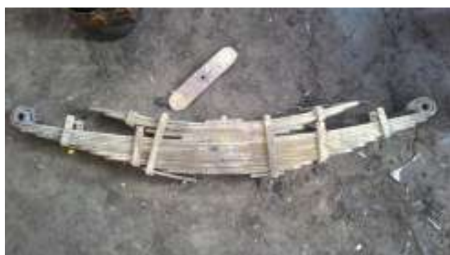
Fig. 7-failure due to bending effect on leaf spring
