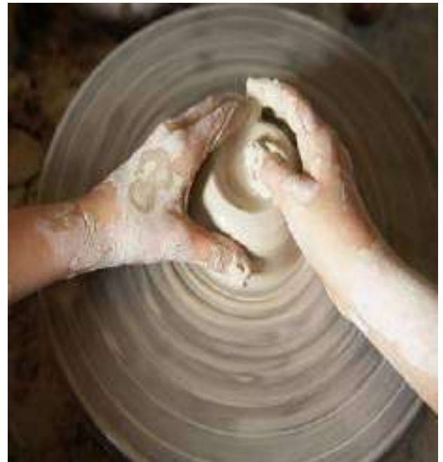
Fig. 2- Centering process in throwing [3]
