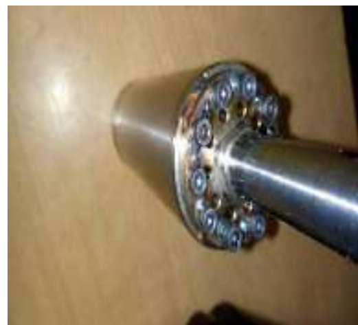
Figure 5 Modification of seat ring and plug in control valve
