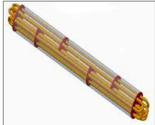
Fig 4. CAD model of shell and tube condenser
