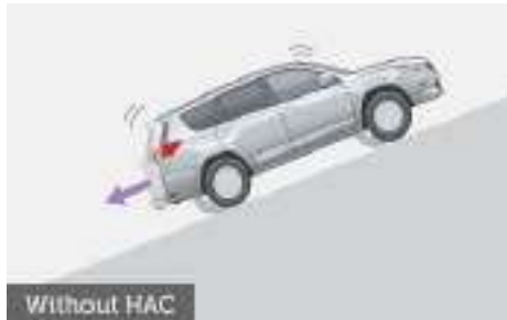
Fig. 2-Ac hill start Assist control
