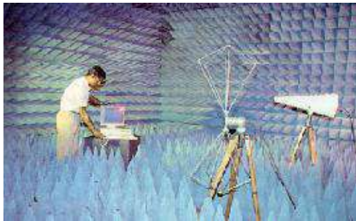
Fig. 3 Radiated Emission testing as per CISPER 11.
